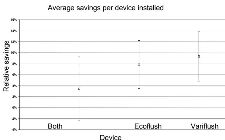
**Figure 14 Average savings per type of device installed**
