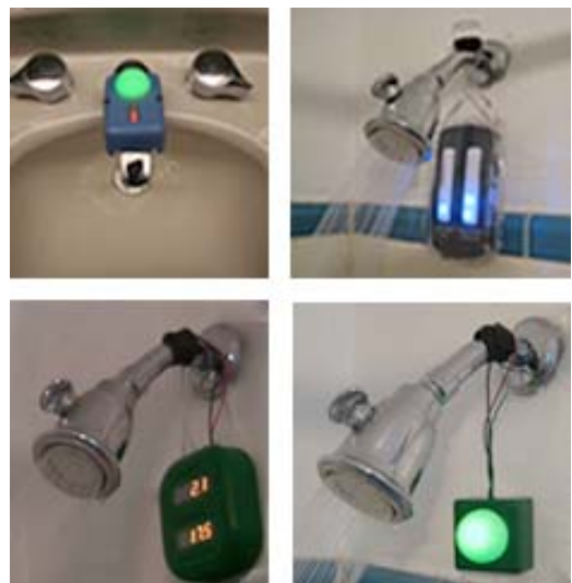
Figure 1. Persuasive displays designed, and deployed in field studies: public faucet display, pilot shower display, numeric shower display, and ambient shower display.
