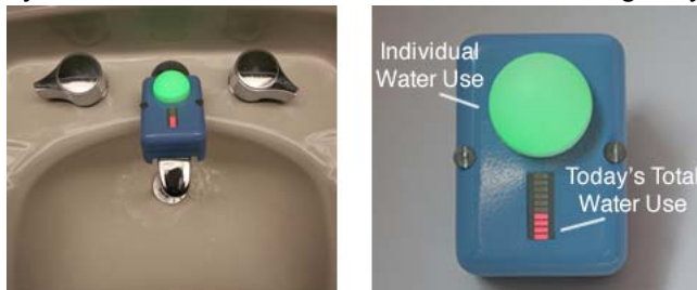
Figure 3. Faucet display mounted onto a public bathroom faucet (left) and each part of the display labeled (right).
